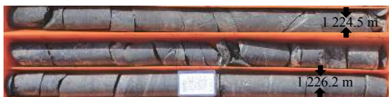
图 5 鼓地 1 井高家边组岩心 LM2—LM5 之间破碎带 Fig.5 A fracture zone between LM2 to LM5 zones of the Kaochiapien Formation found in well GD-1
